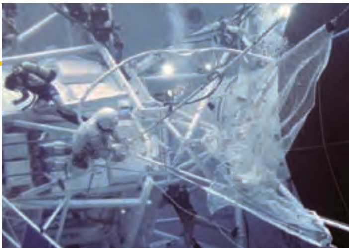
After Skylab's launch, the large, delicate, meteoroid shield on the outside of the workshop was ripped off by the vibration of the launch. Engineers worked frantically to develop solutions to this and other problems and designed a protective solar sail to cover the workshop. Here astronauts practice deploying the protective solar sail in Marshall Space Flight Center's Neutral Buoyancy Simulator. Astronauts Conrad and Kerwin were able to complete the needed repairs to Skylab, salvaging the entire program.
