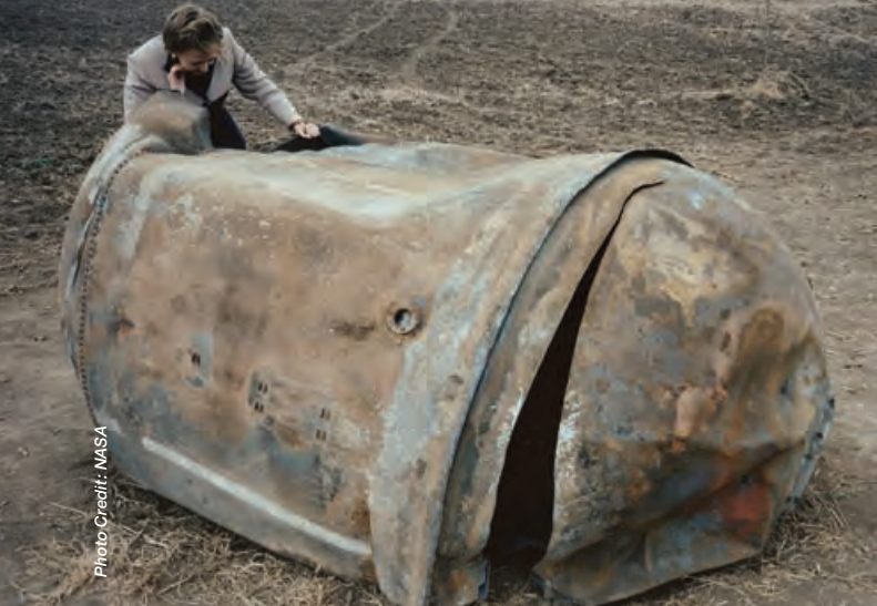
The main propellant tank of the second stage of a Delta 2 launch vehicle landed near Georgetown, Texas, on January 22, 1997. This approximately 250 kg tank is primarily a stainless steel structure and survived reentry relatively intact.
