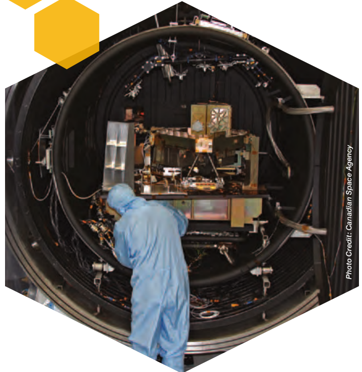
A technician prepares the Canadian-built fine-guidance sensor's engineering test unit for cryogenic testing at the Canadian Space Agency's David Florida Lab in Ottawa.
