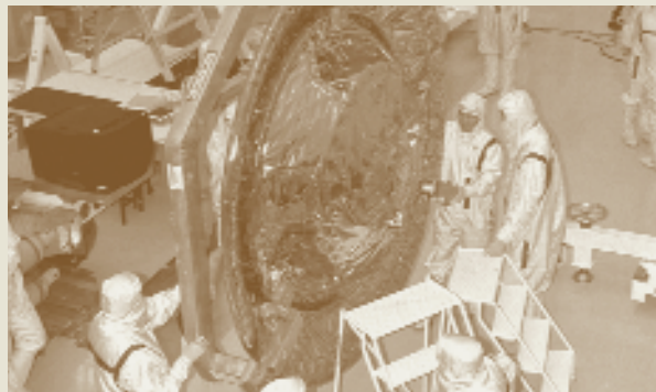
Technicians install the Huygens probe on the Cassini orbiter in the Payload Hazardous Servicing Facility.
