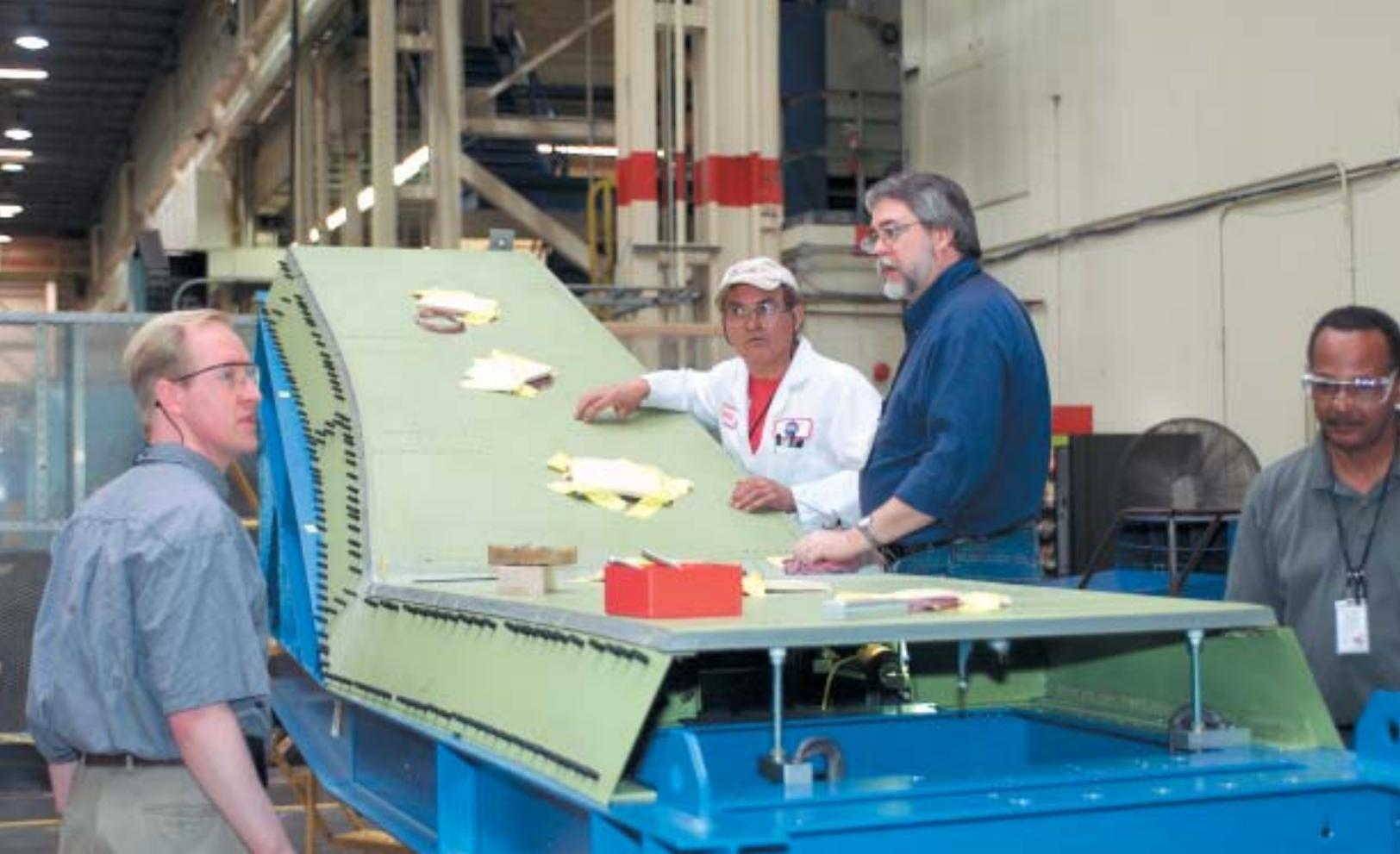
*Technicians at the Johnson Space Center in Houston team up to assemble a test article to simulate the inboard leading edge of a Space Shuttle wing as part of the Columbia Accident Investigation Board's testing.*
