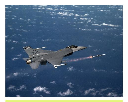
An F-16C Fighting Falcon from the 416th Flight Test Squadron, Edwards Air Force Base, California, launches an advanced medium-range air-to-air missile (AMRAAM) over a Navy test range.
