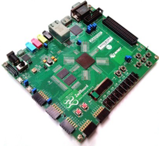
ZedBoard™ is a complete development kit for designers interested in exploring designs using the Xilinx Zynq®-7000 All Programmable SoC.
