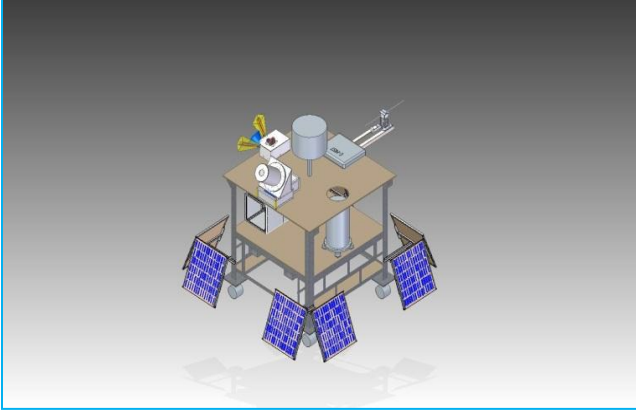
Figure 4: Gondola Configuration, with E-MIST installed on top
