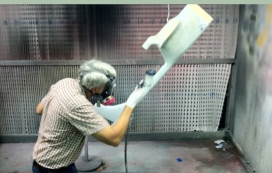
Figure 4. David McLaughlin of KSC's Prototype Shop applies epoxy primer to Genesis fuselage
