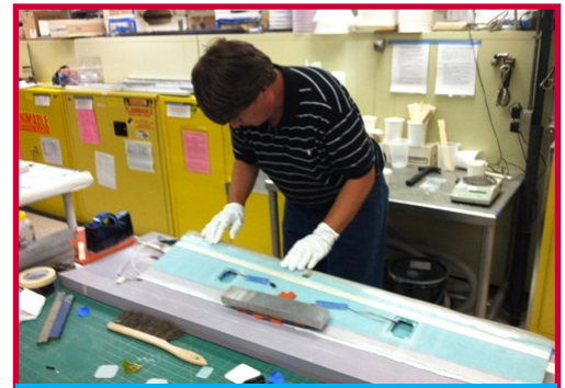
Figure 3. Rocket U's Michael Knutson building Genesis composite wing set
