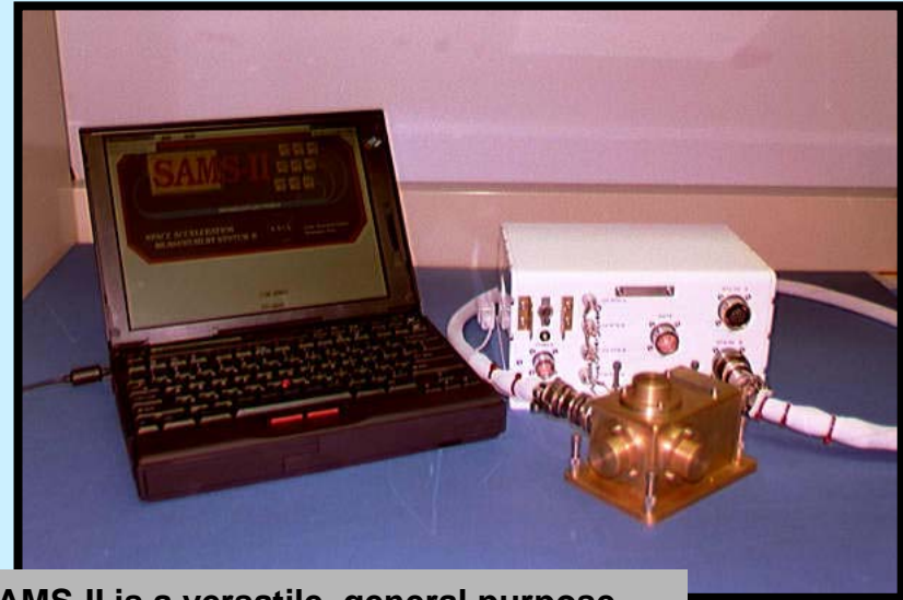
SAMS-II is a versatile, general purpose acceleration measurement system
