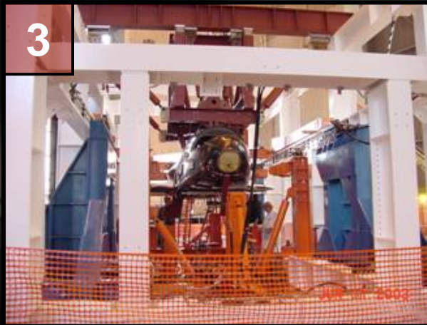
Install Airframe into Test Fixture
