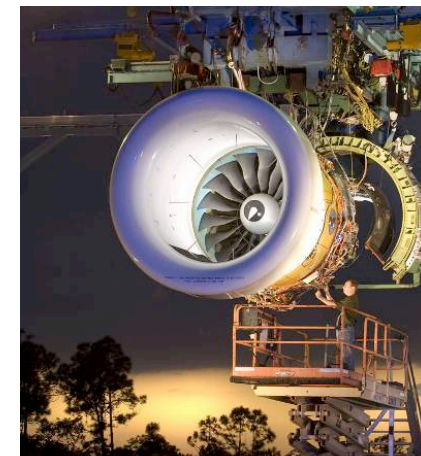
GTF Demonstrator Engine ground test
