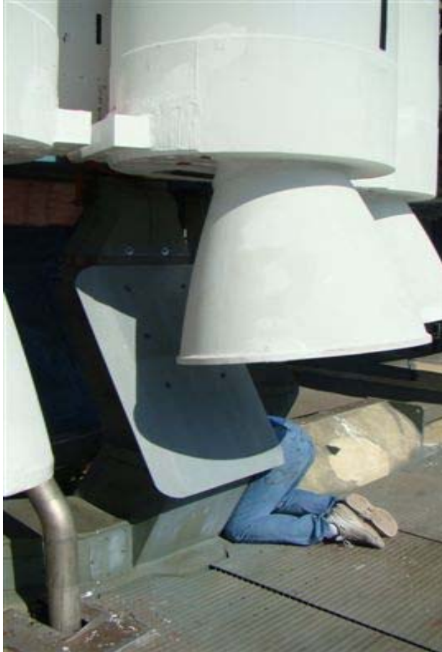
100% Zinc metallize on removable heat shield
