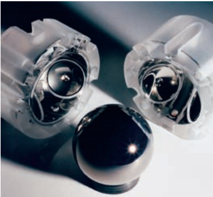
Image of a coated gyroscope rotor and matching housings.
