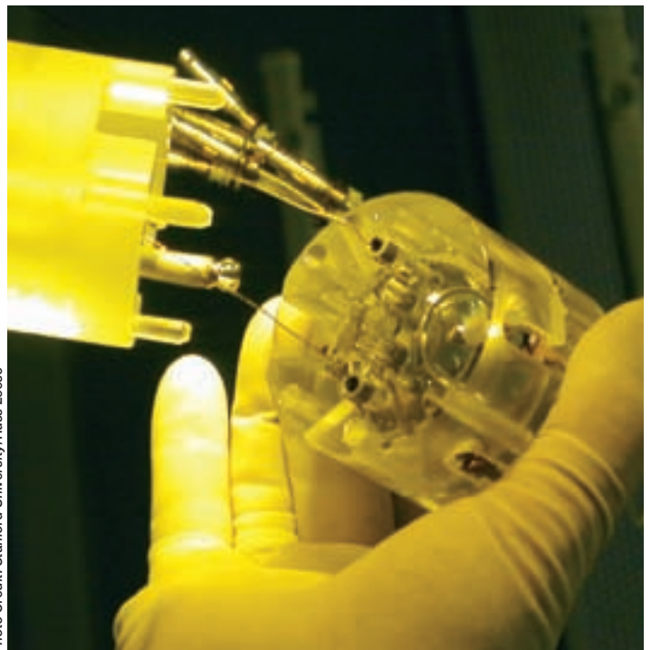
Stanford engineer Chris Gray inspects the number-four gyro under monochromatic light after it was removed from the Science Instrument assembly.
