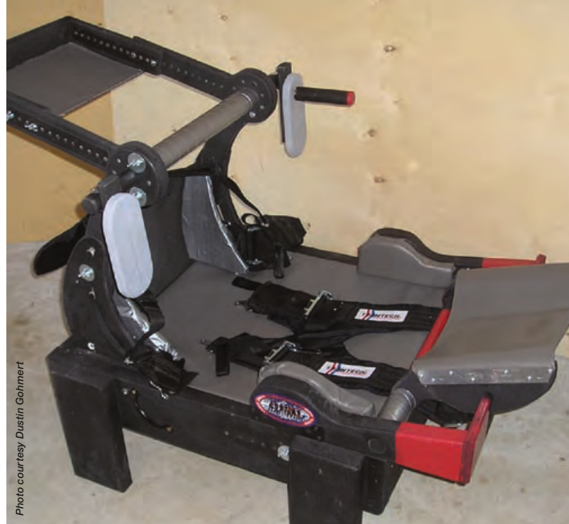
Isometric view of the seat adjusted to accommodate 99th percentile operator.
