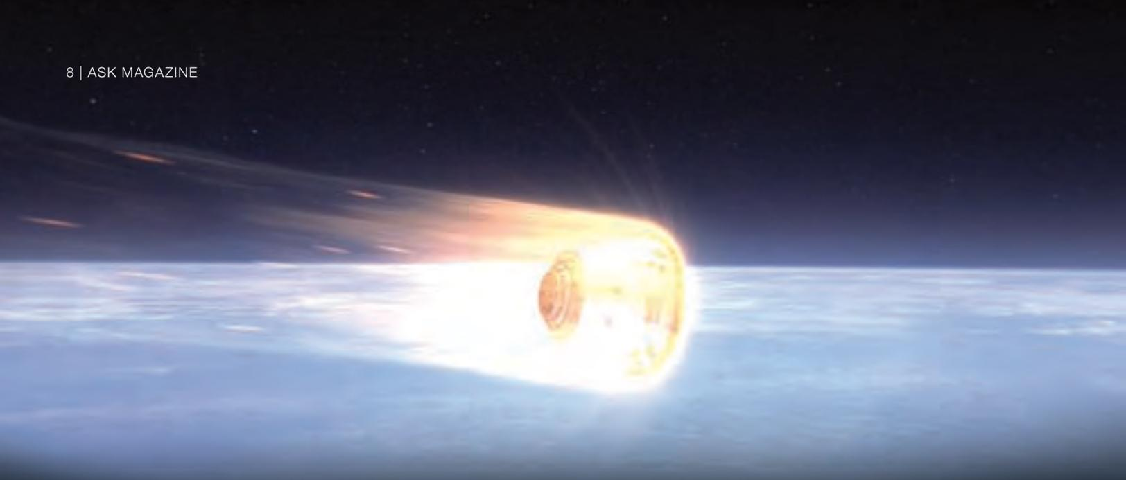
*Protected by a PICA-X heat shield in this artist's rendition, the Dragon spacecraft reenters the earth's atmosphere at around 7 kilometers per second (15,660 mph), heating the exterior of the spacecraft as high as 2,000°C (3,620°F).*
