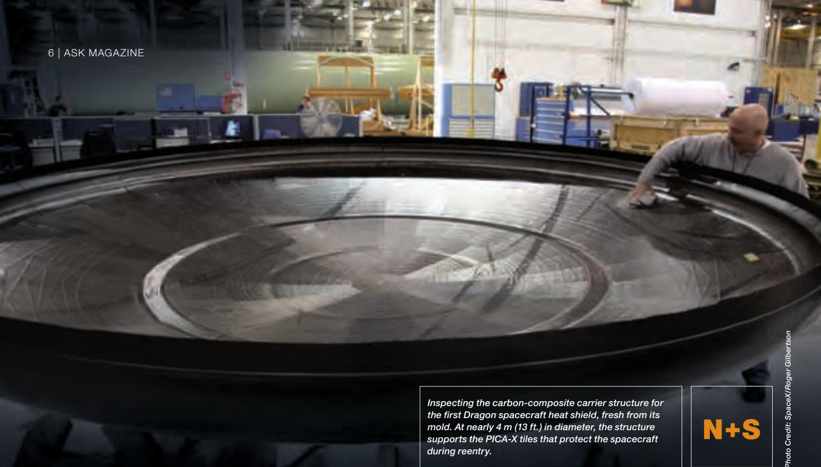
*Inspecting the carbon-composite carrier structure for the first Dragon spacecraft heat shield, fresh from its mold. At nearly 4 m (13 ft.) in diameter, the structure supports the PICA-X tiles that protect the spacecraft during reentry.*
