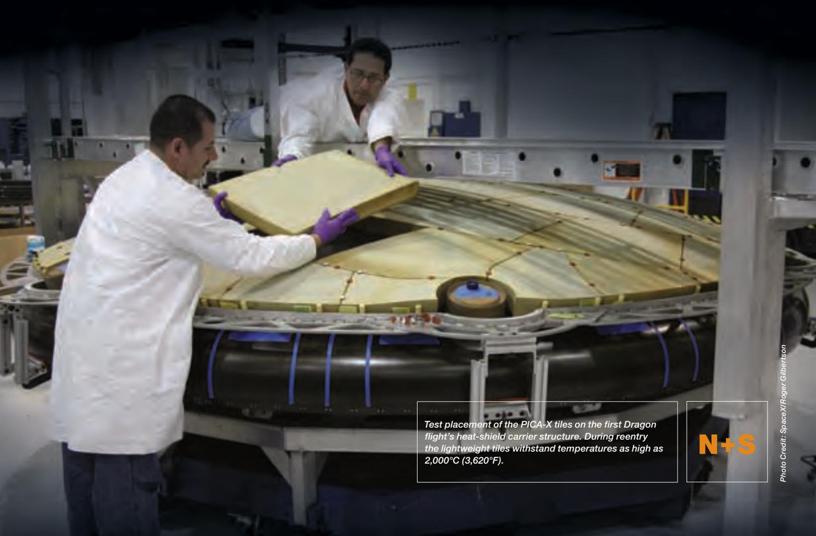
*Test placement of the PICA-X tiles on the first Dragon flight's heat-shield carrier structure. During reentry the lightweight tiles withstand temperatures as high as 2,000°C (3,620°F).*
