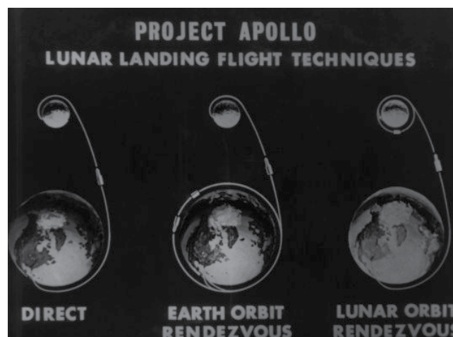
The three principal contending lunar landing techniques: direct ascent (left), earth-orbit rendezvous (center), and lunar-orbit rendezvous (right). Credit: NASA
