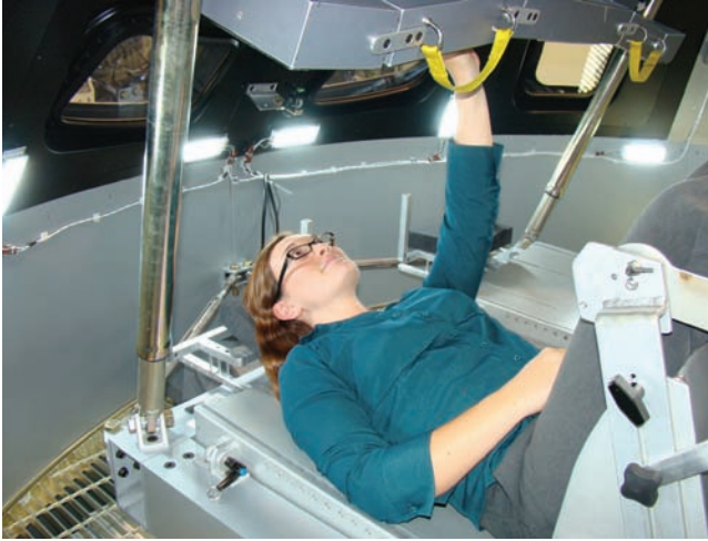
Kat Coderre in the Human Engineering Structural Mockup. This full-scale Orion mockup is used for crew evaluations such as ergonomic assessments and emergency egress operations. Photo Credit: Lockheed Martin
