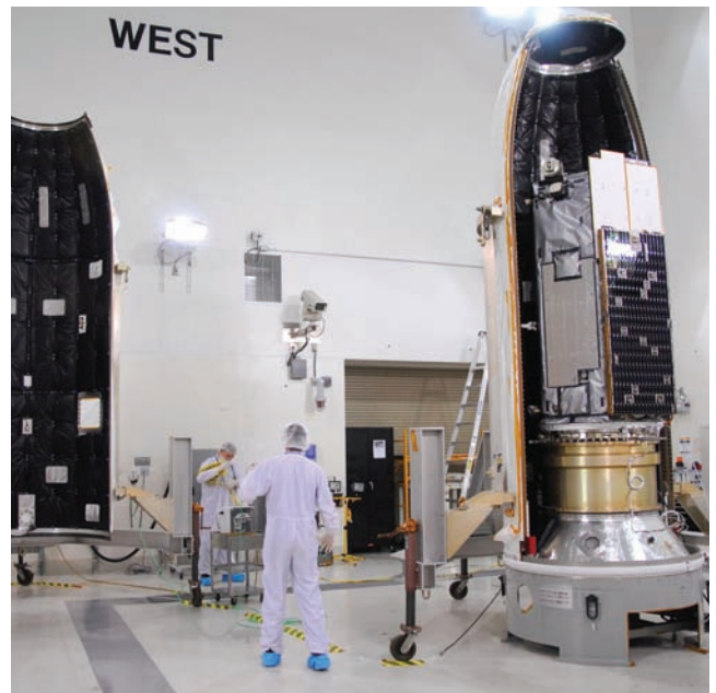
Inside Building 1032 at Vandenberg Air Force Base, technicians install the Orbiting Carbon Observatory spacecraft inside the payload fairing. Photo Credit: NASA
