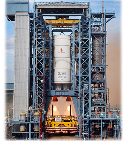
L110 Stage Test at Mahendragiri
