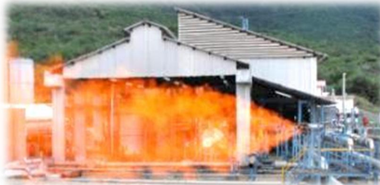
Testing of C25 Turbo pump with GG & Startup system
