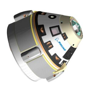
System Description: Commercial crew transportation system comprises the reusable CST-100 spacecraft, launch services, and ground systems. CST-100 is compatible with multiple launch vehicles and is reusable for up to ten missions.
