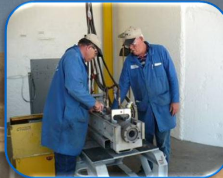
5 Inch Propellant Center Perforated Subscale Testing
