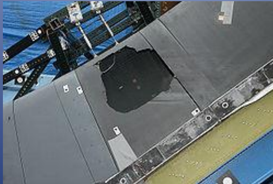
RCC panel foam impact test
