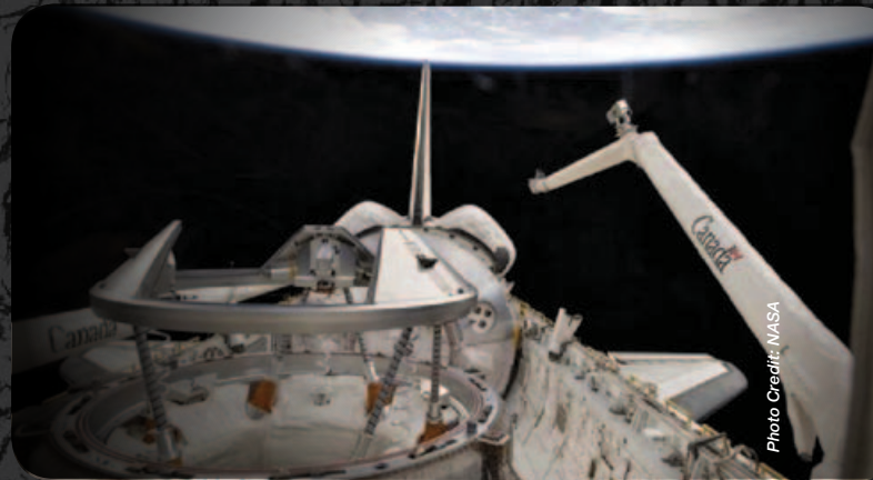
The shuttle capture ring ready to dock with station during STS 131.
