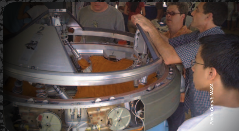
Visitors learn about the docking mechanism that allows the Space Shuttle to dock with the International Space Station.
