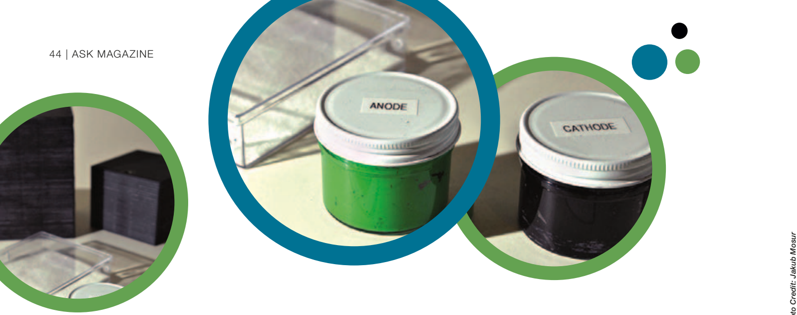
Ceramic fuel cells coated with special inks are at the core of the Bloom Energy Server.
