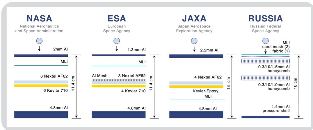
**Figure 2.5.1 NASA, JAXA, ESA, and Russia's levels of protection on ISS.**
