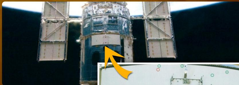
**Image 1.1.1** Particle impact features on the Hubble Space Telescope.
