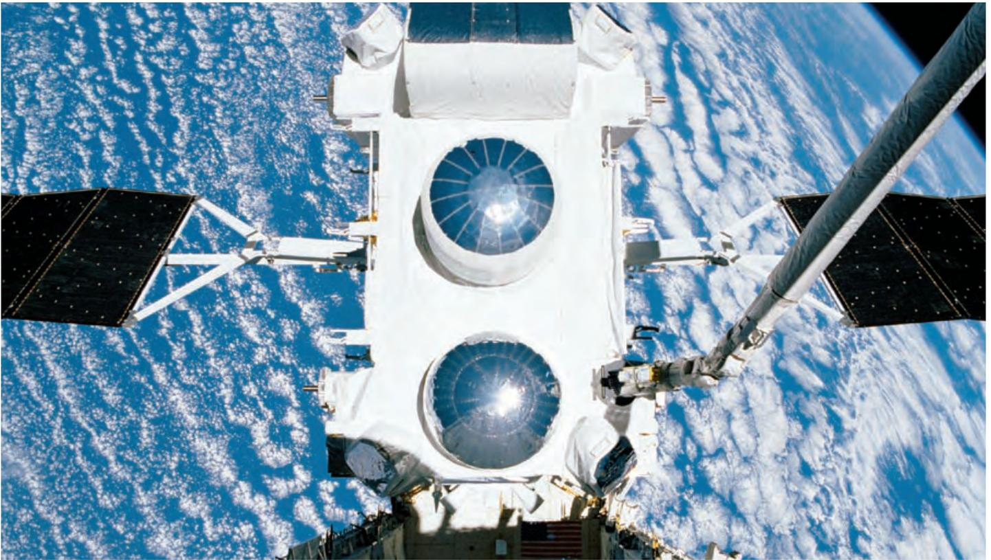
*The Gamma Ray Observatory (GRO) with its solar array panels deployed is grappled by the remote manipulator system April 11, 1991. This view taken by the STS 37 crew shows the GRO against a backdrop of clouds over water on the Earth's surface.*
