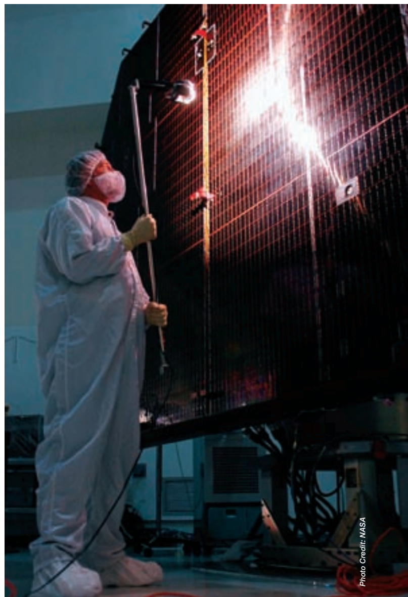
A technician at Astrotech in Titusville, Fla., conducts an illumination test on the Deep Impact spacecraft as a final check of performance.
