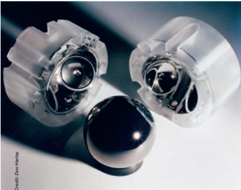
Image of a coated gyroscope rotor and matching housings.
