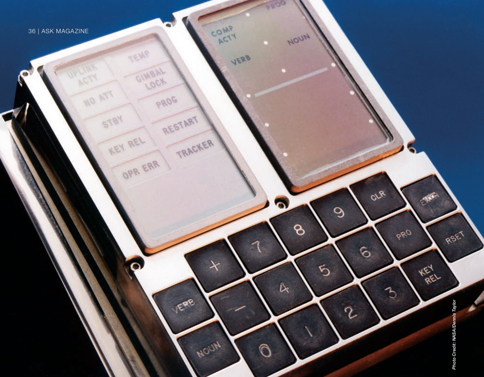
The Apollo Display Keyboard Assembly (DSKY) used on the lunar module.
