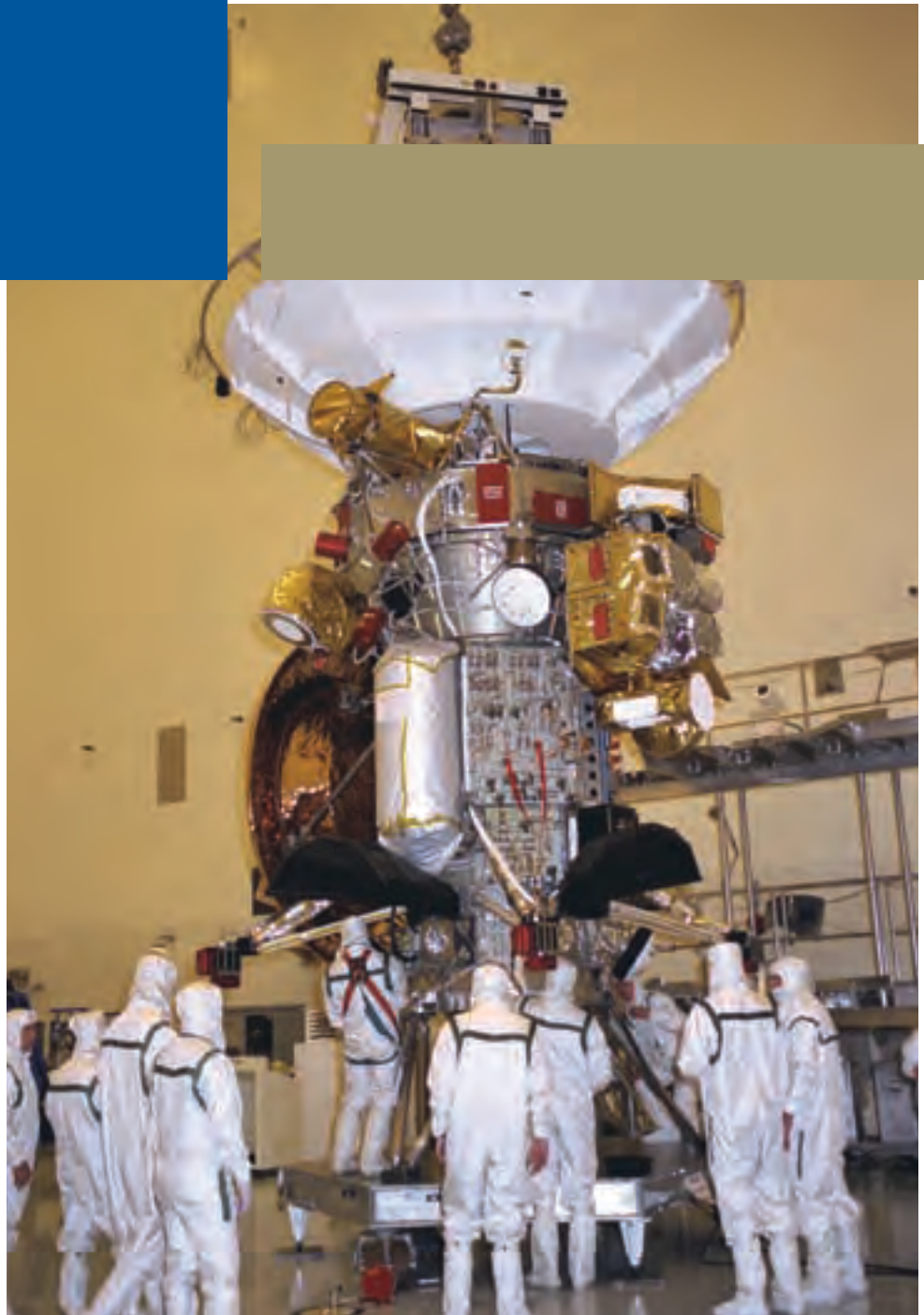
The Cassini spacecraft is mated to the launch vehicle adapter in Kennedy Space Center's Payload Hazardous Servicing Facility. Cassini was once frequently cited as an example of what NASA should not do because of its size, complexity, and cost.
