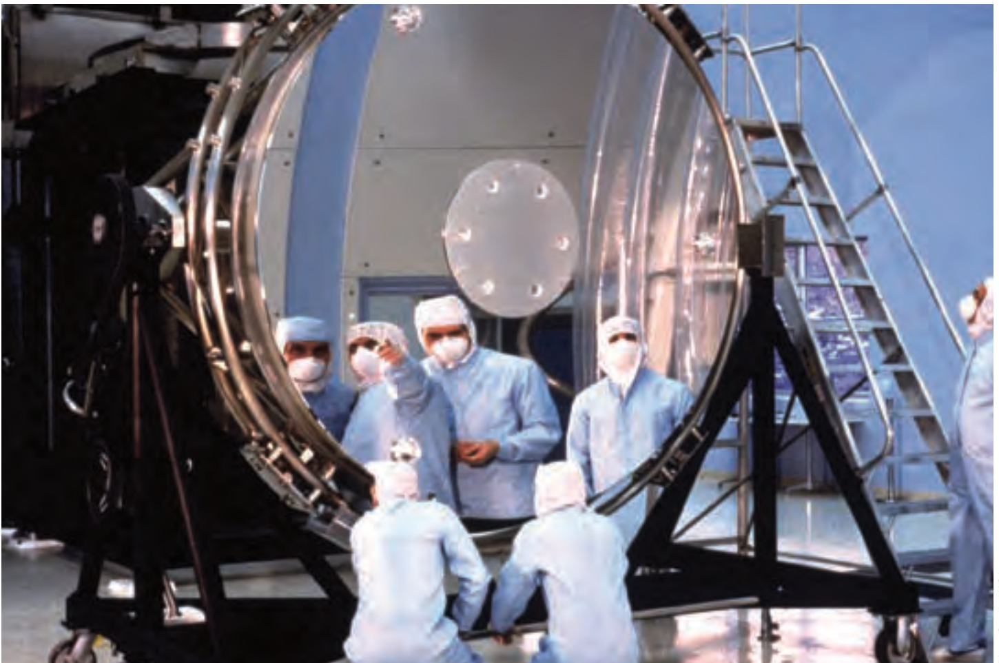
Workers study Hubble's main, eight-foot (2.4 m) mirror. The flaw in the Hubble Space Telescope's optics was due in part to reductions in testing to save money.
