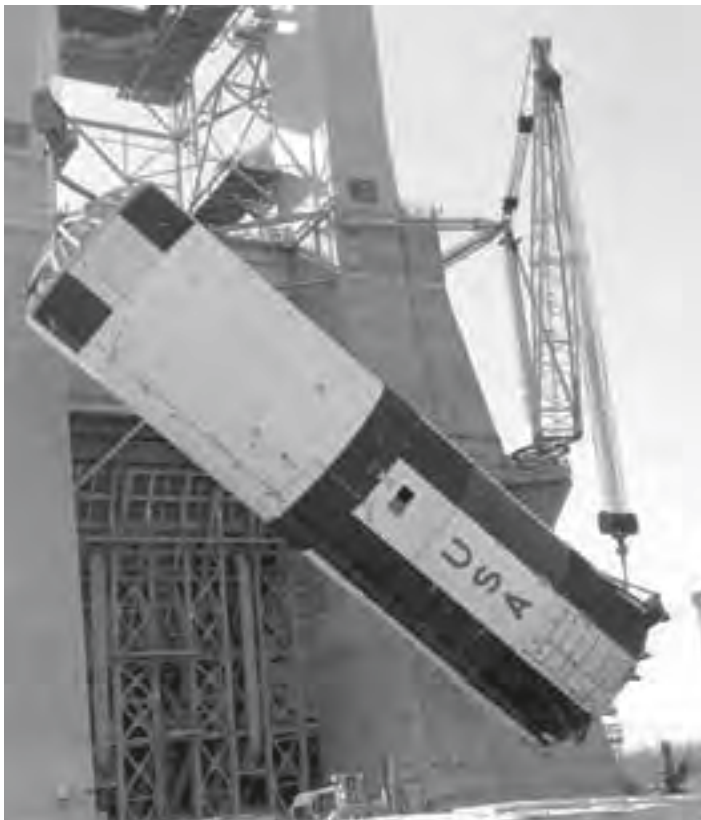
The 138-foot-long first stage of the Saturn V is lowered to the ground following a successful static test firing at Marshall Space Flight Center's S-1C test stand.
