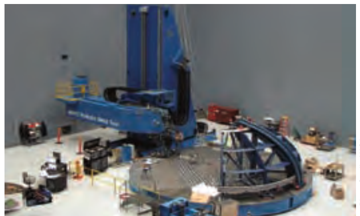
This robotic weld tool at Marshall Space Flight Center is configured to assemble the domes at the ends of each of the Ares I Upper Stage propellant tanks.
