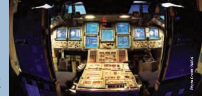
This "fish-eye" view shows NASA's Multifunction Electronic Display Subsystem (MEDS), otherwise known as the "glass cockpit." The fixed-base Space Shuttle mission simulator in the Johnson Space Center's Mission Simulation and Training Facility was outfitted with MEDS to be used by flight crews for training.
