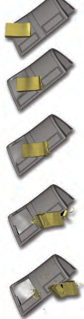
Comparison of the LS-DYNA predictions with high-speed video of the full-scale test.
