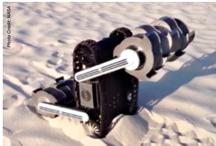
With a pair of drums positioned on arms, RASSOR can take on a number of different shapes to accomplish its work.
