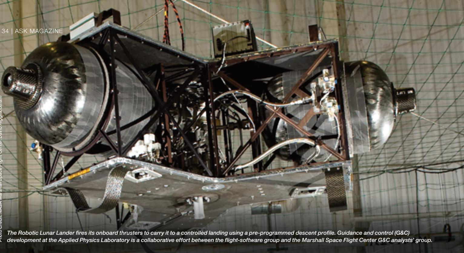
The Robotic Lunar Lander fires its onboard thrusters to carry it to a controlled landing using a pre-programmed descent profile. Guidance and control (G&C) development at the Applied Physics Laboratory is a collaborative effort between the flight-software group and the Marshall Space Flight Center G&C analysts' group.
