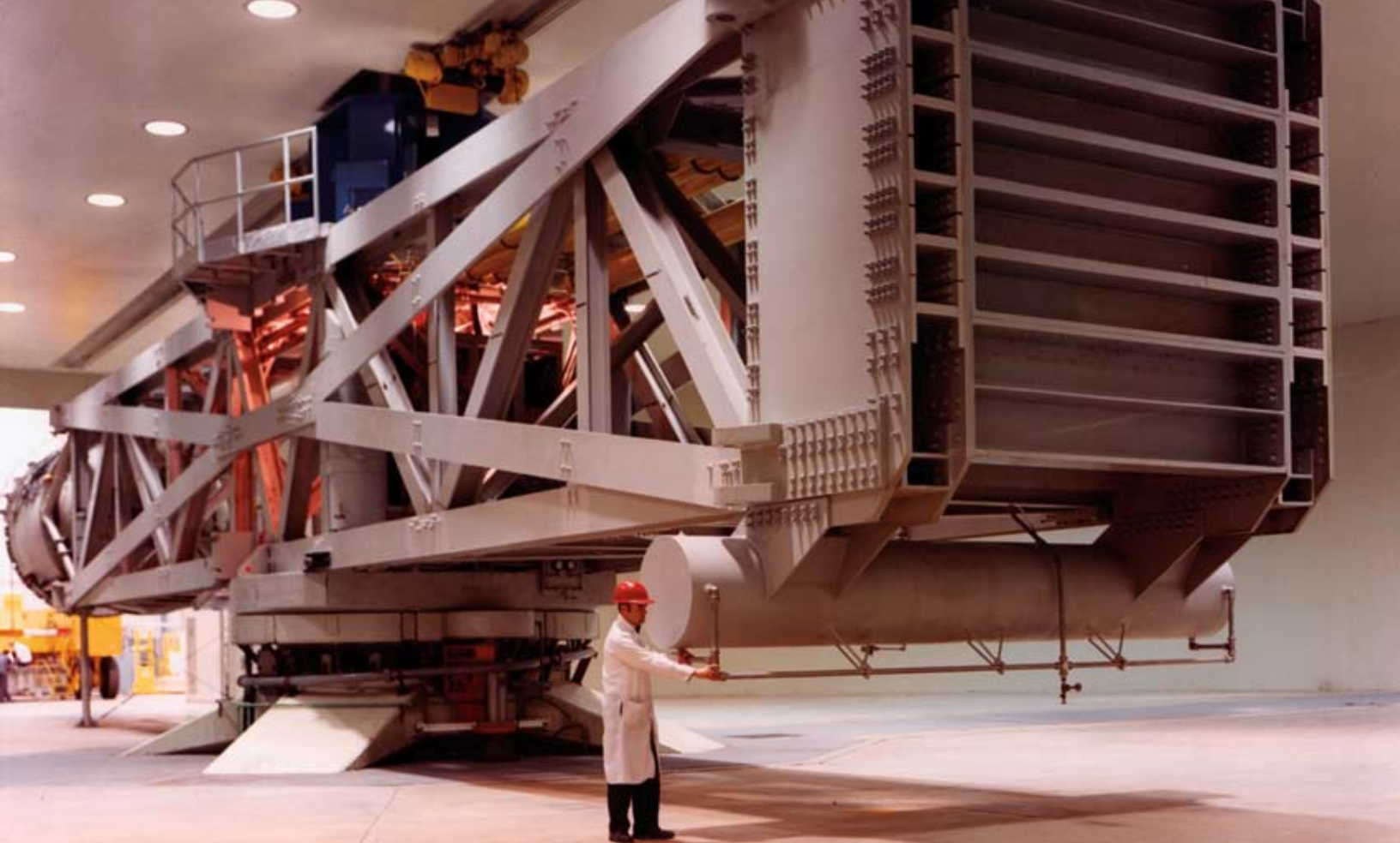
Goddard Space Flight Center's launch phase simulator.
