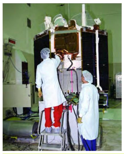
The John Hopkins Applied Physics Laboratory in Columbia, Maryland had responsibility for building the Advanced Composition Explorer (ACE) spacecraft. Scientific instruments were mounted on the outisde of the spacecraft, providing workers with easy access when they had to be removed following the integration and testing phase of the project.
