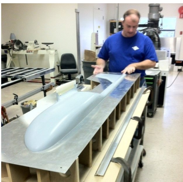
Figure 2: Luke Catella places parting plane template at KSC's Prototype Shop in June 2013.
