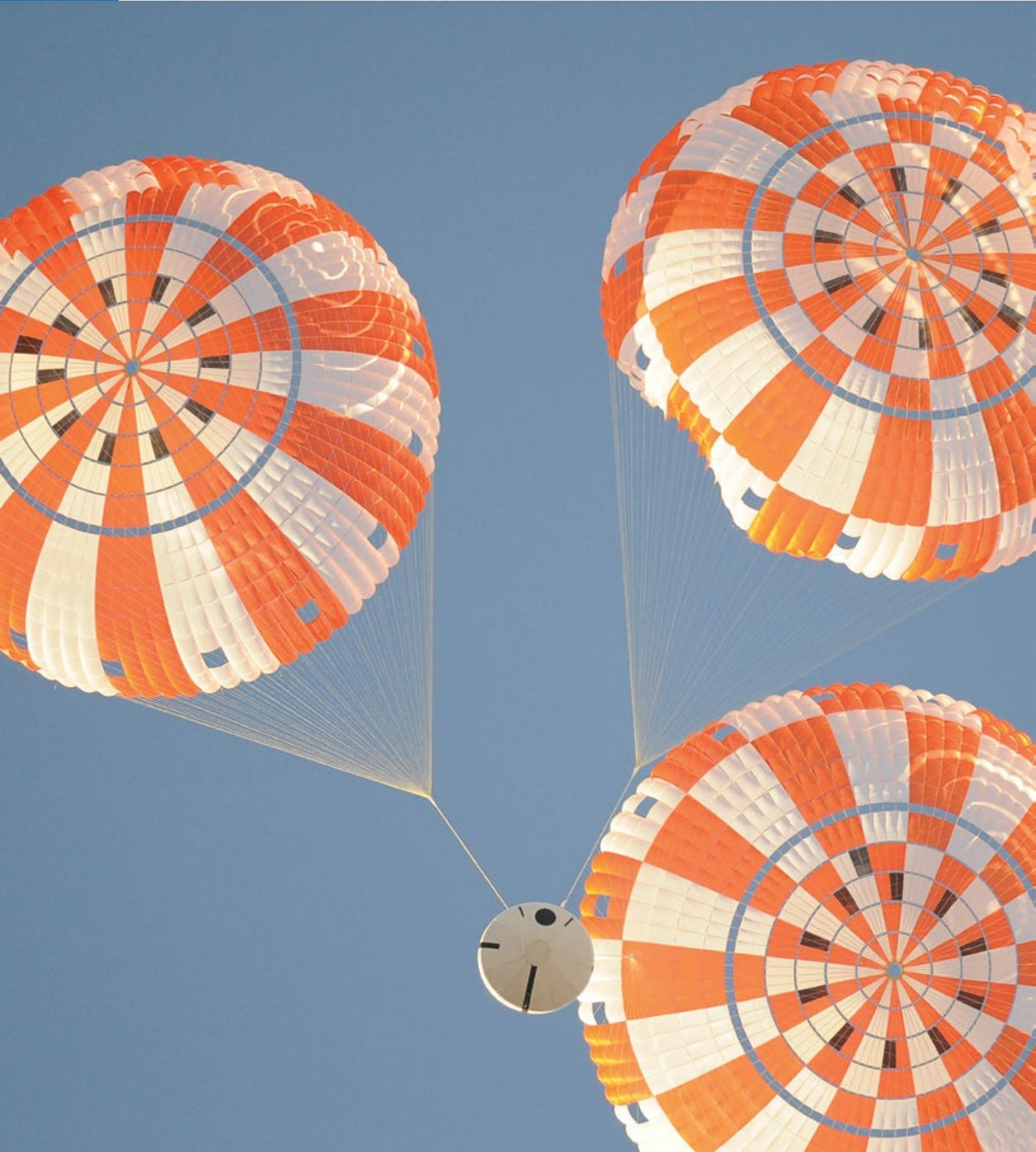
Orion Capsule Parachute Assembly System (CPAS) drop test using the Parachute Test Vehicle (PTV) at the Yuma Army proving grounds in Arizona.
