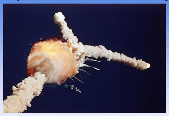
**Proximate cause**: O-rings turn brittle in cold weather.
