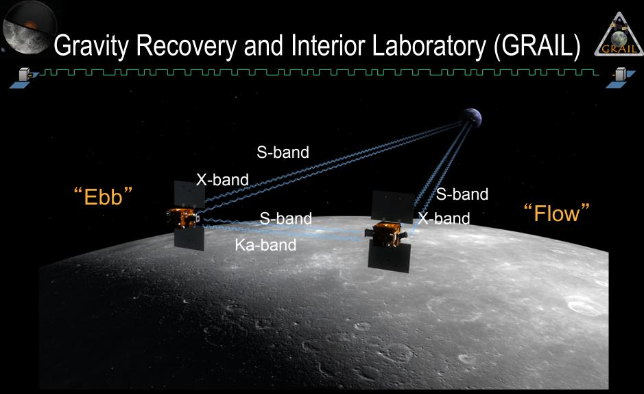
GRAIL is a 2-spacecraft mission that senses the Moon's gravity field by measuring the change in distance between 2 spacecraft 60 to 225 km apart in the same ~55 km altitude orbit for a period of ~3 months. The Extended Mission added ~3 months of mapping at 25-75 km distance @ an average altitude of 23 km. The Endgame added 10 days of mapping @ an average altitude of 11 km.
