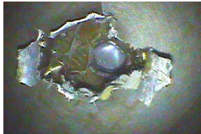
Radiator damage caused to space shuttle Endeavour by MMOD impact during STS-118 in 2007.
