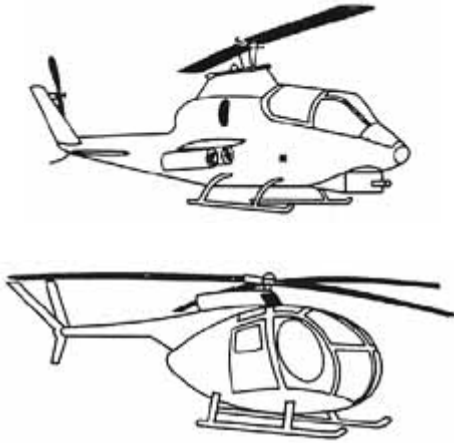
(a) Bell AH-1G Huey Cobra. Two-bladed. (b) Hughes OH-6A. Four-bladed.
