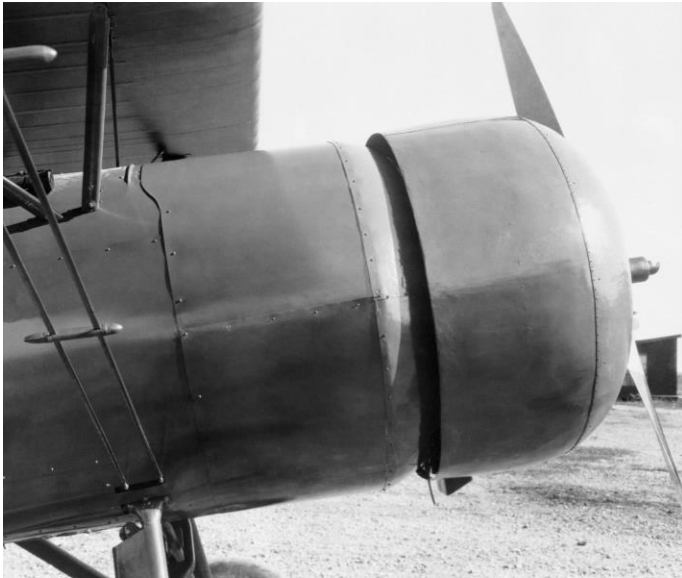
The NACA Cowling “Engineering Science” The NACA until WWII
