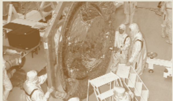
Technicians install the Huygens probe on the Cassini orbiter in the Payload Hazardous Servicing Facility.
